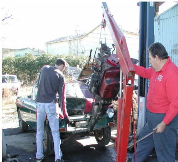
Bob Thompson removing the engine of a 1970 MGB
